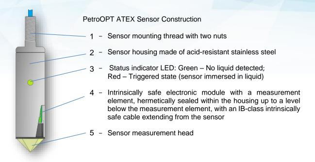
Inside the sensor, there is an electronic module that is hermetically sealed with potting material and connected to a cable. The cable is oil-resistant, designed for intrinsically safe systems, and shielded. It contains three numbered black conductors:
